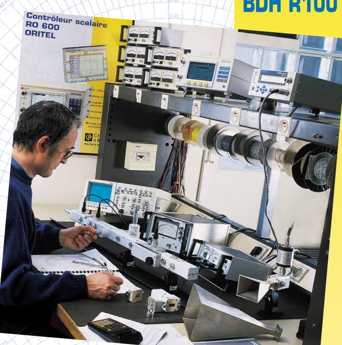
Made up of a set of components which are sturdy and very easy to implement, the ORITEL BDH 100 bench enables a great many basic microwave experiments to be conducted.
